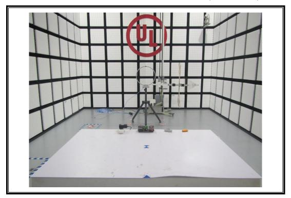
RADIATED EMISSIONS MEASUREMENT SETUP (Below 30MHz)
