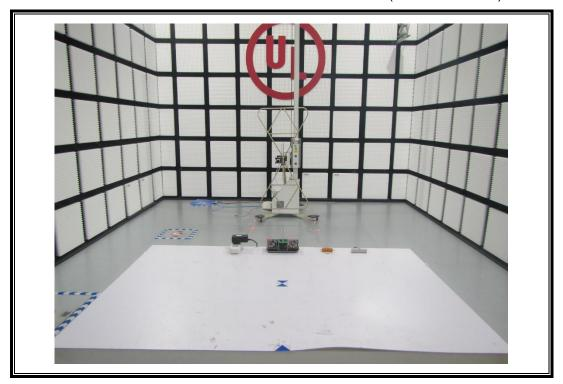
RADIATED EMISSIONS MEASUREMENT SETUP (30MHz  $\sim$  1 GHz)
