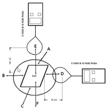
Note1: As bottom point is not required to test for desktop devices, so we scanning all the surfaces and recorded the worst level in F.
