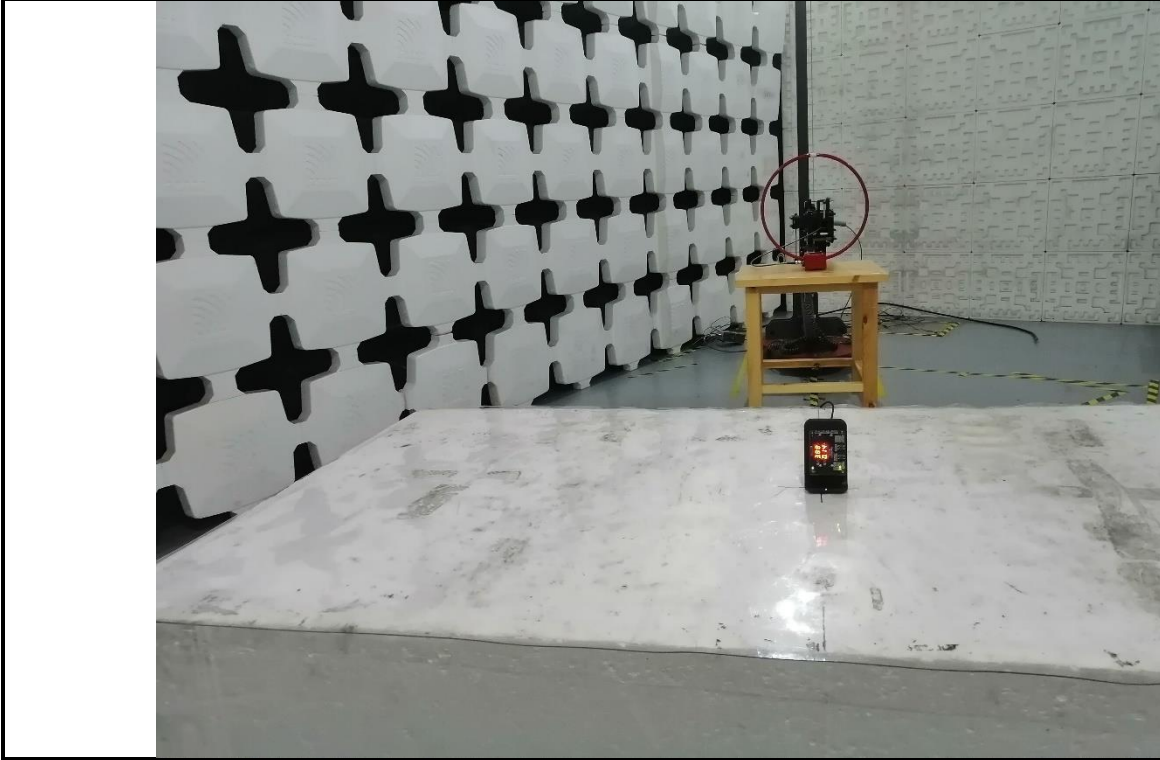
Radiated emission Test Setup (Below 30MHz)
