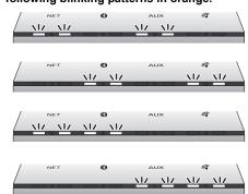
There is a problem with this unit. Disconnect the AC power supply cord from the AC outlet, reconnect it to the AC outlet after about 30 seconds. If the problem still persists, disconnect the AC power supply cord and consult your dealer
