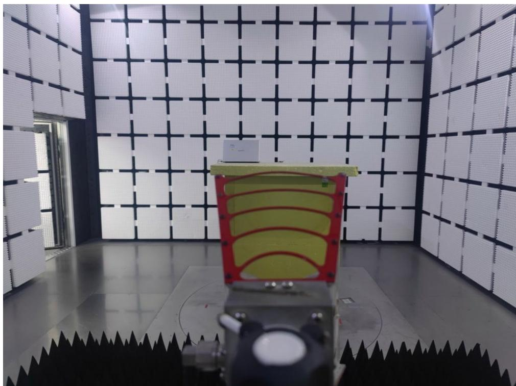
**Radiated Emissions Test Photos****Above 1 GHz\_Harmonic (18 GHz to 26.5 GHz)**
