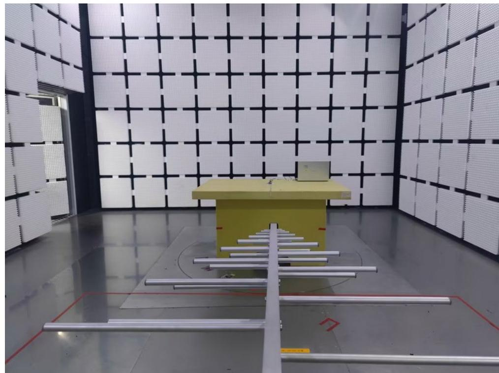
**Radiated Emissions Test Photos****Above 1 GHz\_Band edge & Harmonic (1 GHz to 18 GHz)**
