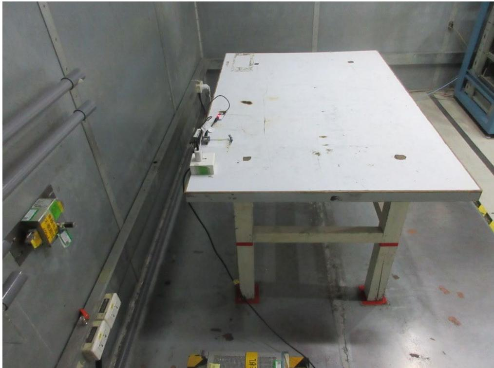
**Radiated Emissions Test Photos****9 kHz to 30 MHz**
