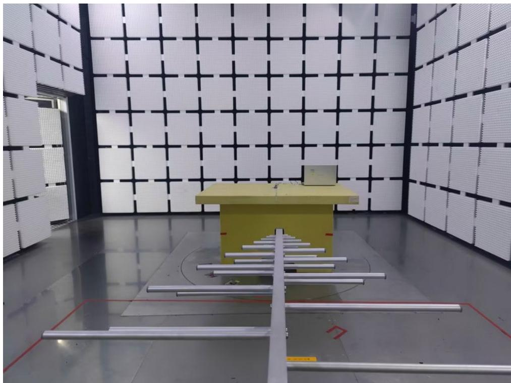
**Radiated Emissions Test Photos****Above 1 GHz\_Band edge & Harmonic (1 GHz to 18 GHz)**
