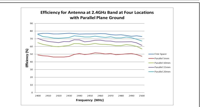
FIGURE 6.3.4 EFFICIENCY OF ANTENNA AT 2.4GHZ BAND AT FOUR LOCATIONS WITH PARALLEL PLANE GROUND
