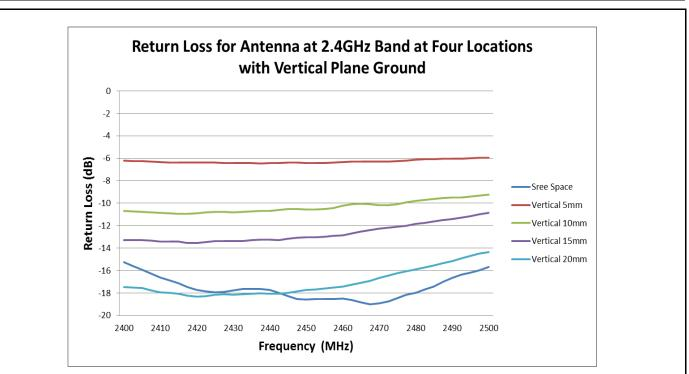
FIGURE 6.2.2 RETURN LOSS OF ANTENNA AT 2.4GHZ BAND AT FOUR LOCATIONS WITH VERTICAL PLANE GROUND
