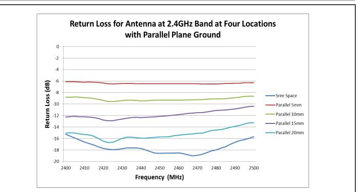
FIGURE 6.3.2 RETURN LOSS OF ANTENNA AT 2.4GHZ BAND AT FOUR LOCATIONS WITH PARALLEL PLANE GROUND
