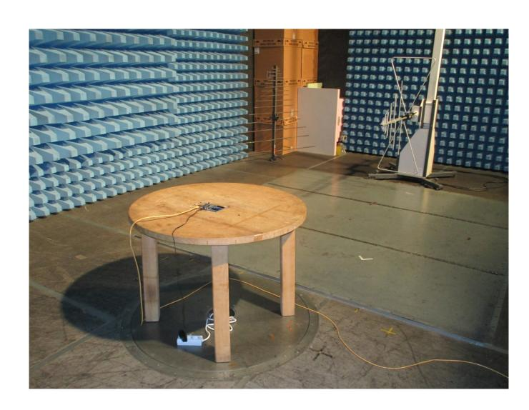
Description: Test setup above 1 GHz
