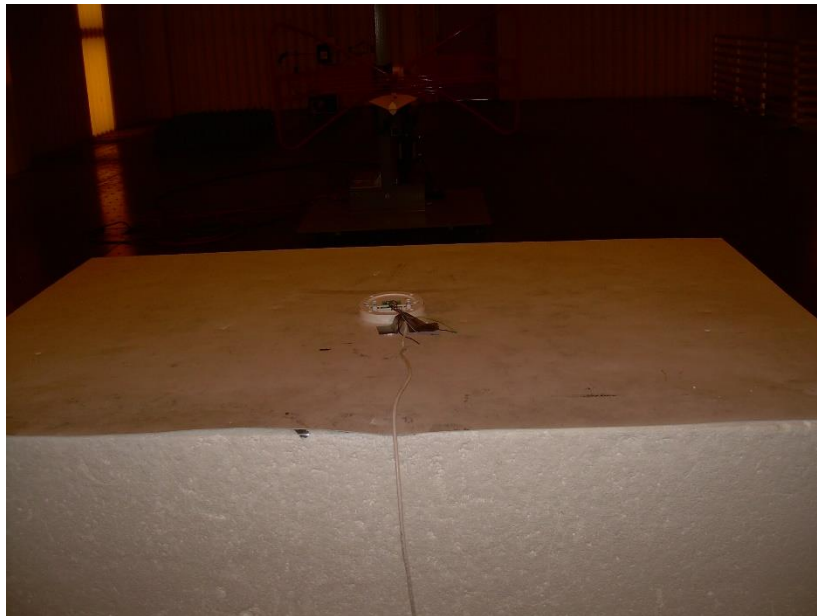
Photograph 2: Back View Radiated Emissions Worst-Case Configuration – 30 – 1000 MHz
