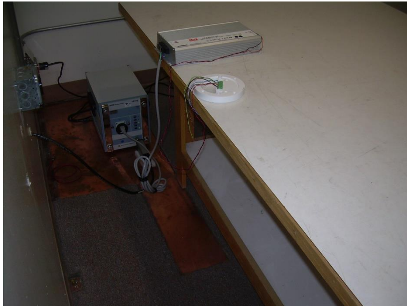
Photograph 6 – Back View Conducted Emissions Worst-Case Configuration
