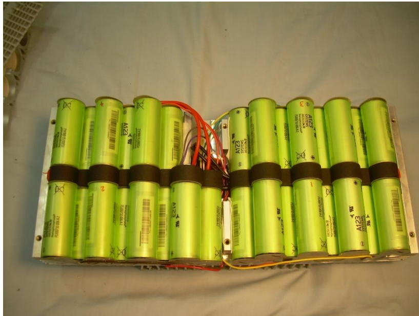
Photograph 12 – Internal View of the EUT Battery Pack
