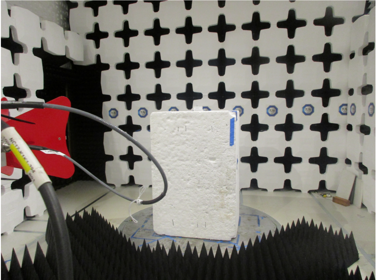
Figure 6: Radiated Band-Edge Emissions – Front View – above 1 GHz
