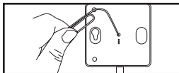
Figure 8.3 - Press and release the recessed button on the bottom of the bridge
