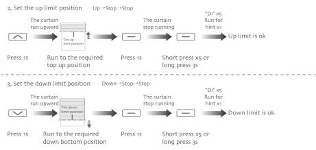
Note:The motor power off, then re-power on, the motor will exit the limit settings mode; Unfinished limit setting withdrew from limiy position setting mode, if setting before have limit then continue to use the previous limit
