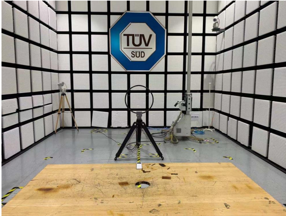
Radiated Emission Setup 9kHz ~ 30MHz
