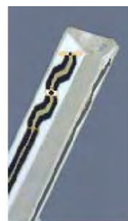
Figure 3.3 Probe Thick-Film Technique
