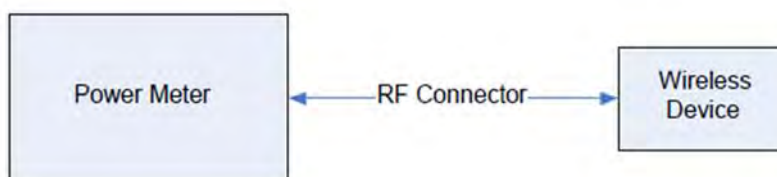
Figure 8.1.1 Power Measurement Setup
