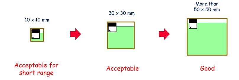
If installed on a small PCB, connecting PCB's ground to the common ground of the unit is preffered because total ground can be seen larger.
