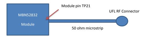
The design of the 50 ohm microstrip on the customer's PCB is crucially important. Compliant operation of the MBN is dependent on proper construction of this 50 ohm line and the following guidelines must be followed to ensure legal operation of the product. The diagram below shows the required microstrip structure to be routed between module pin TP21 and the UFL connector.
