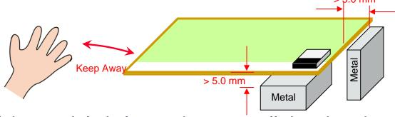
If the module is located on a small daughter board, please make ground connected strongly and regard ground plane including entire main board.
