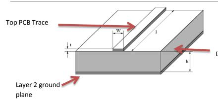
Note the representative dimensions shown in the drawing above. It is imperative that the module customer (the integrator) use the exact dimensions we recommend to ensure a 50 ohm impedance for this transmission line.
