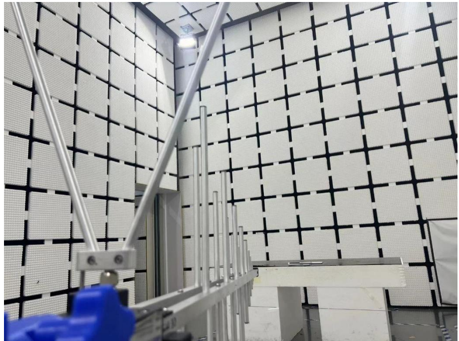
Radiation Emission Test Setup (30MHz to 1GHz)
