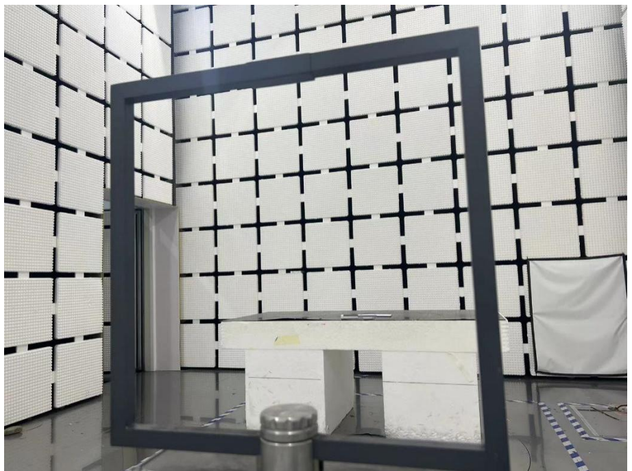
Radiation Emission Test Setup (Below 30MHz)
