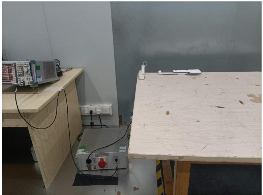
Conducted Emission Test Setup
