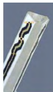
Figure 3.3 Probe Thick-Film Technique
