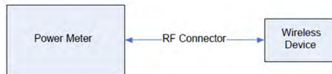
Figure 8.1.1 Power Measurement Setup
