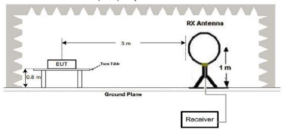
(2) Radiated Emission Test-Up Frequency 30MHz~1GHz
