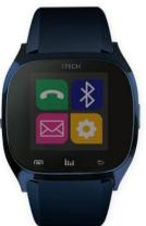
**Power Key**: Power On/Off ; Awaken/turn off screen ; Back to main menu **Touch screen**: Each function (main menu) will be shown and displayed on capacitive touch screen.
