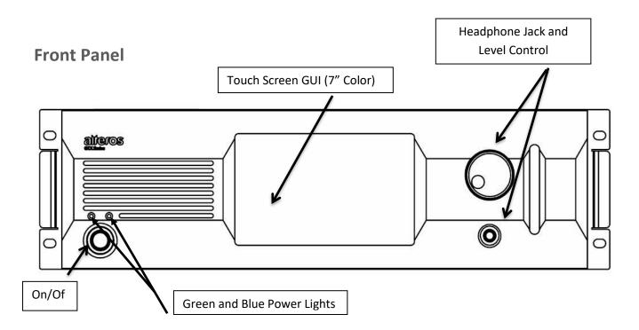
The Front Panel design has minimal controls; the majority of Monitoring and control are handled through the touchscreen GUI. If a channel is selected using the GUI its audio will be routed to the headphone jack and VU meter.
