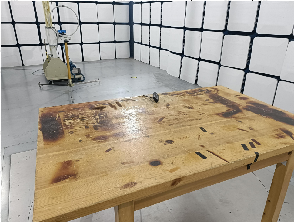
Photo of Radiation Emission Test (below 30MHz)
