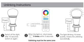
Unlinking must be the same zone with the Linking If the light not blink quickly, the unlink failed, pls switch off the light again, and follow the above steps to unlink again.
