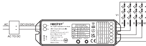
Controller connect to RGB+CCT LED strip diagram
