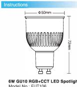
GW GU10 RGB+CCT LED Spotlight Model No.: FUT106 Voltage: 100-240V~ 50/60Hz Rated Current: 0.11A Working Temp.:-10~40°C Color Temp.: 2700K~6500K Luminous Efficiency: 90LM/W Luminous Flux: 550LM CRI: >80 PF: 0.55 Lifespan: 50000h Beam Angle: 30° RF: 2.4GHz Control Distance: 30m Product Weight: 69g
