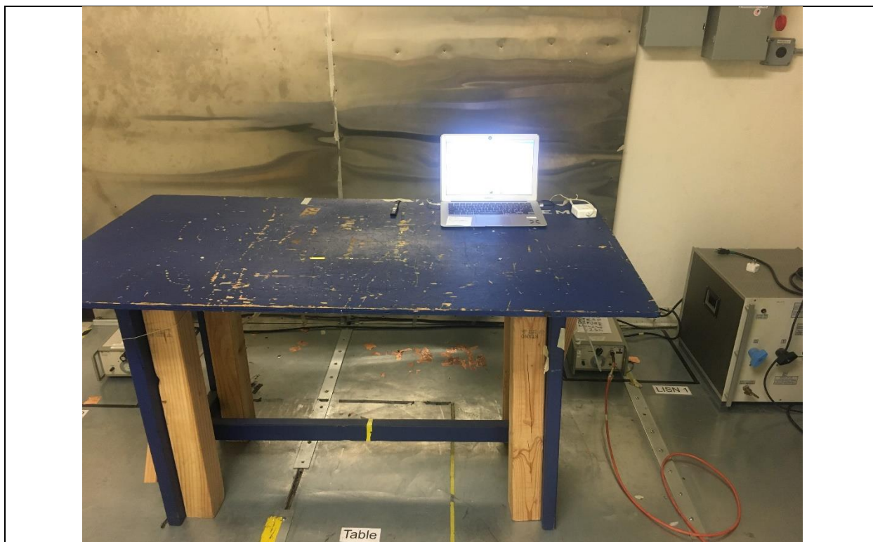
Conducted Emission Test Front View
