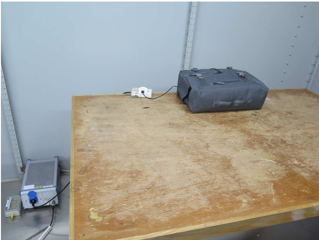
Charging mode (Line-conducted emission)
