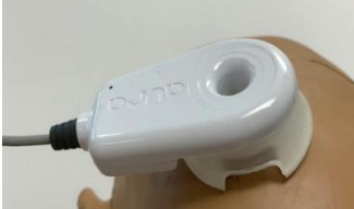
Figure 13: Antenna Holster being affixed onto scalp above AURA™ Sensor.
