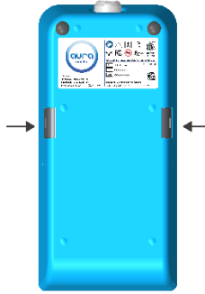
Figure 3: Press locking buttons simultaneously to release battery.
