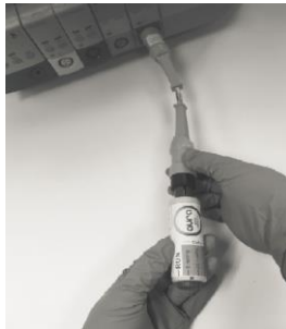
Figure 14: AURA™ Data Receiver connecting into Patient Monitor IBP Port.
