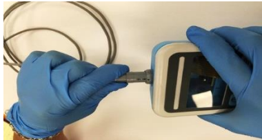
Figure 11: Plug antenna cable into AURA™ Monitor.
