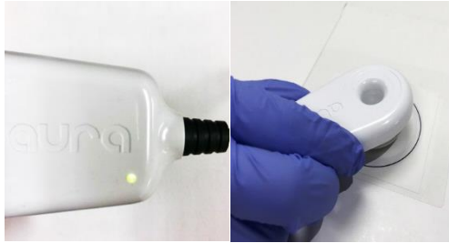
Figure 12: Positioning the AURA™ Antenna at the sticker on the AURA™ Sensor Tray box to run in-package check.
