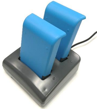
Figure 8: Slide batteries into battery charger.
