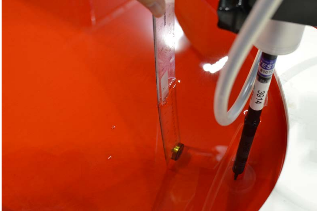
SAR Test Setup Photo 3 – Inactive AURA Sensor in 13MHz Head Liquid with SAR Probe
