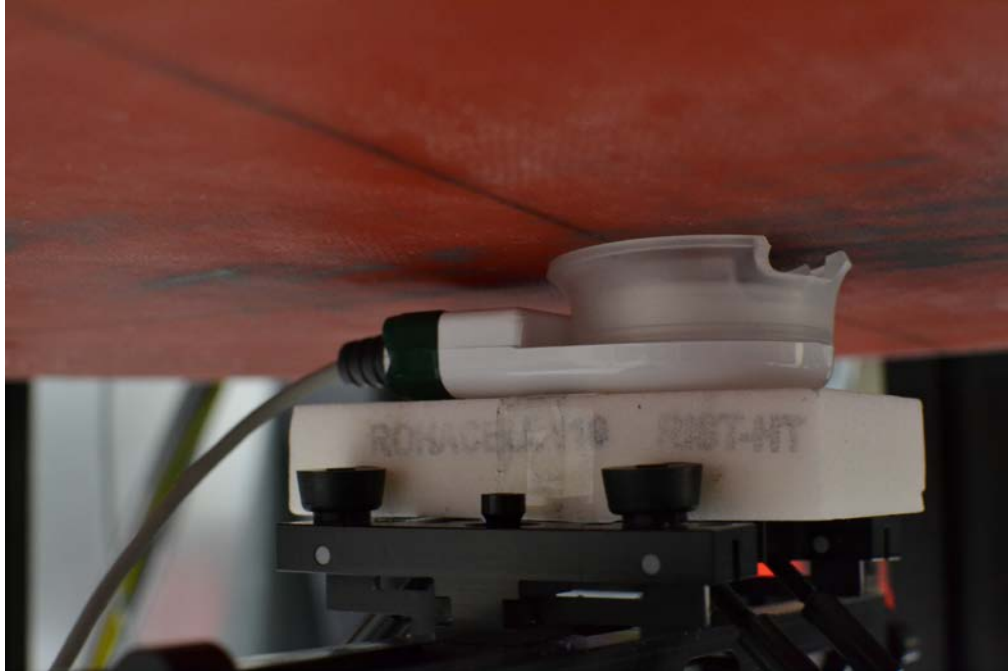
SAR Test Setup Photo 1 – Bottom Edge at 0 mm
