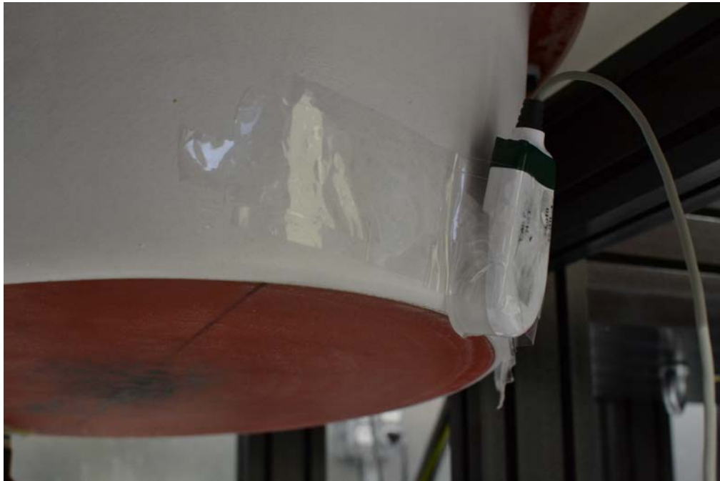
SAR Test Setup Photo 2 – AURA Antenna positioned on side of ELI Phantom
