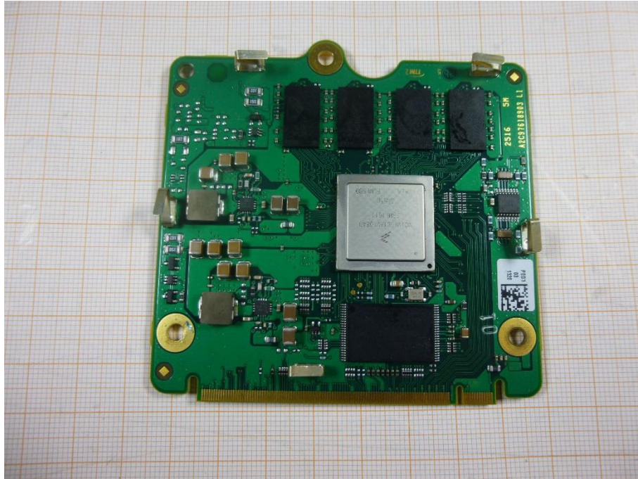
Photo 3: Display Controller detailed front view
