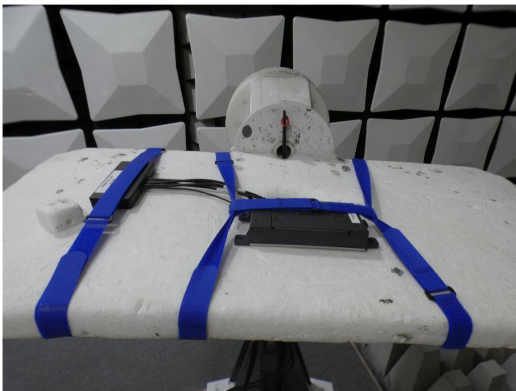
Photo 7: Test setup for radiated measurements, detailed view (1 – 26 GHz; Fully anechoic chamber, FCC Parts 15.247, 22, 24 and 27; ANSI C63.10)
