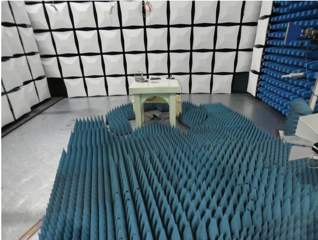
Photo 5: Test setup for radiated measurements (semi-anechoic chamber above 1 GHz; unintentional radiator §15.109, ANSI C63.4)
