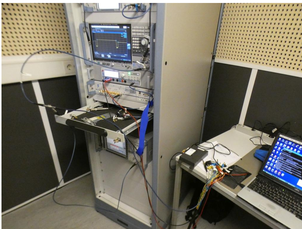
Photo 8: Test setup for conducted measurements (FCC Part 15.247; ANSI C63.10)
