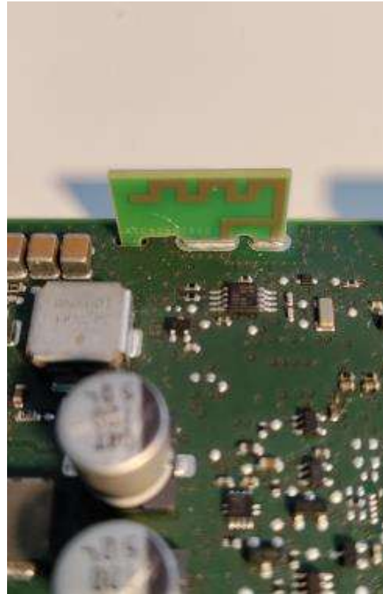
Bluetooth/WiFi antenna Position inside the device (left), Picture of antenna (right)
