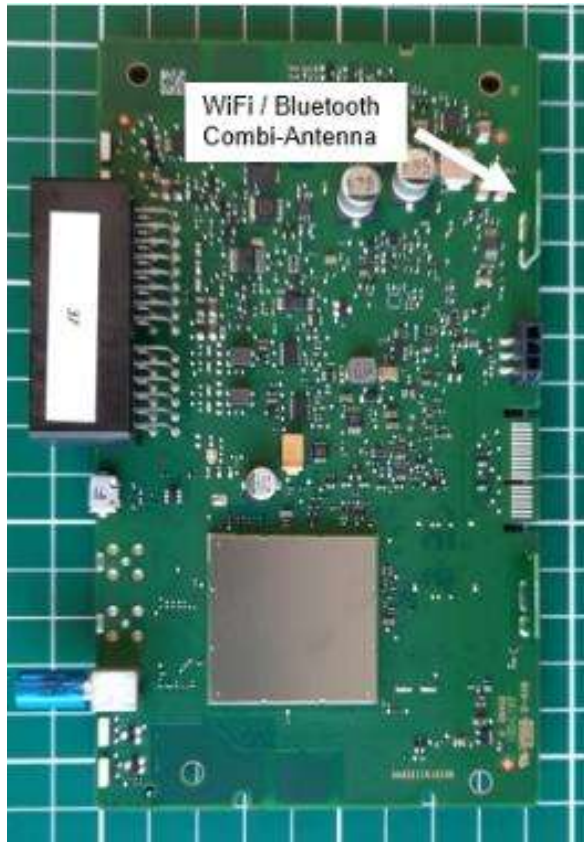
Bluetooth/WiFi antenna Position inside the device (left), Picture of antenna (right)
