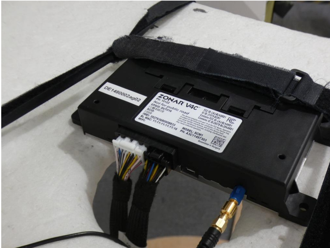
Photo 4: Test setup for radiated measurements, detailed view (standalone setup, 1 GHz – 24 GHz; FCC 15c247)
