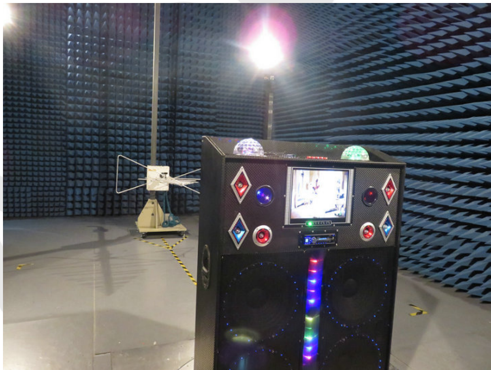
Photo of Radiation Emission Test
