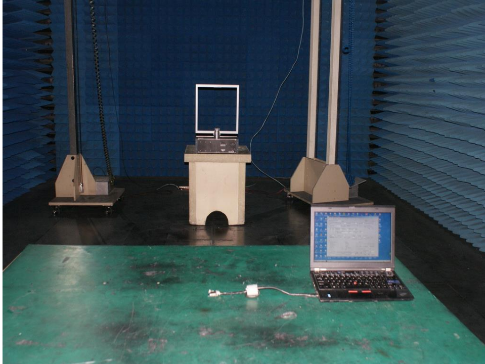
Photograph 2: Set-up for Spurious Emissions (30MHz-1GHz)
