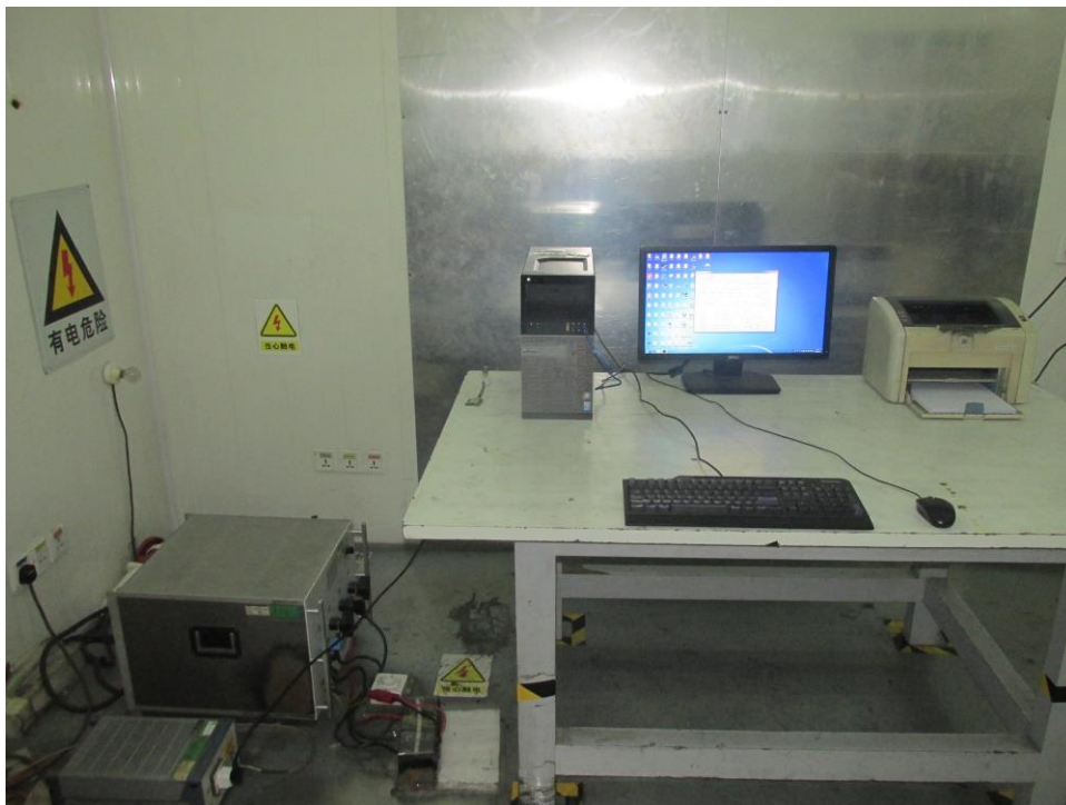
Photograph 6: Setup for Conducted emissions on AC Mains
