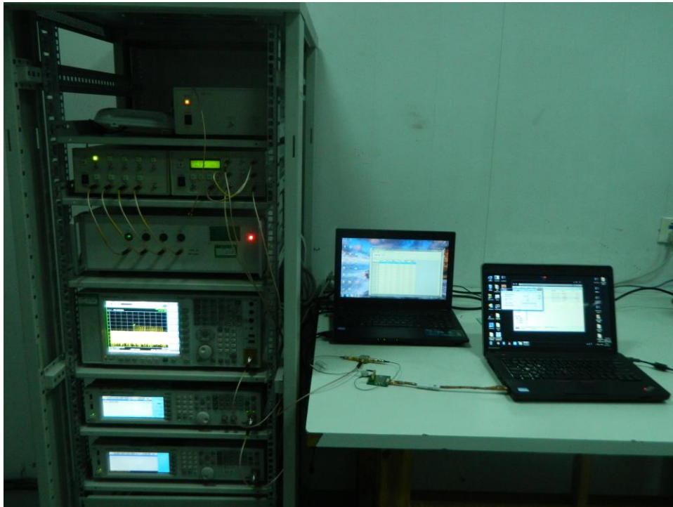
Photograph 2: Setup for Spurious emissions, Below 30MHz
