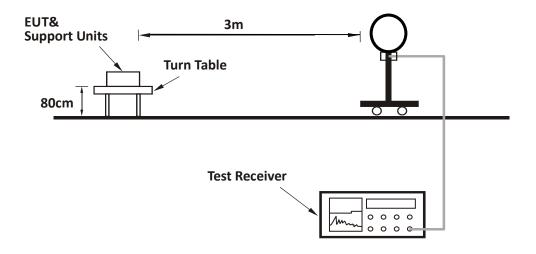
For Radiated emission 30MHz to 1GHz:
