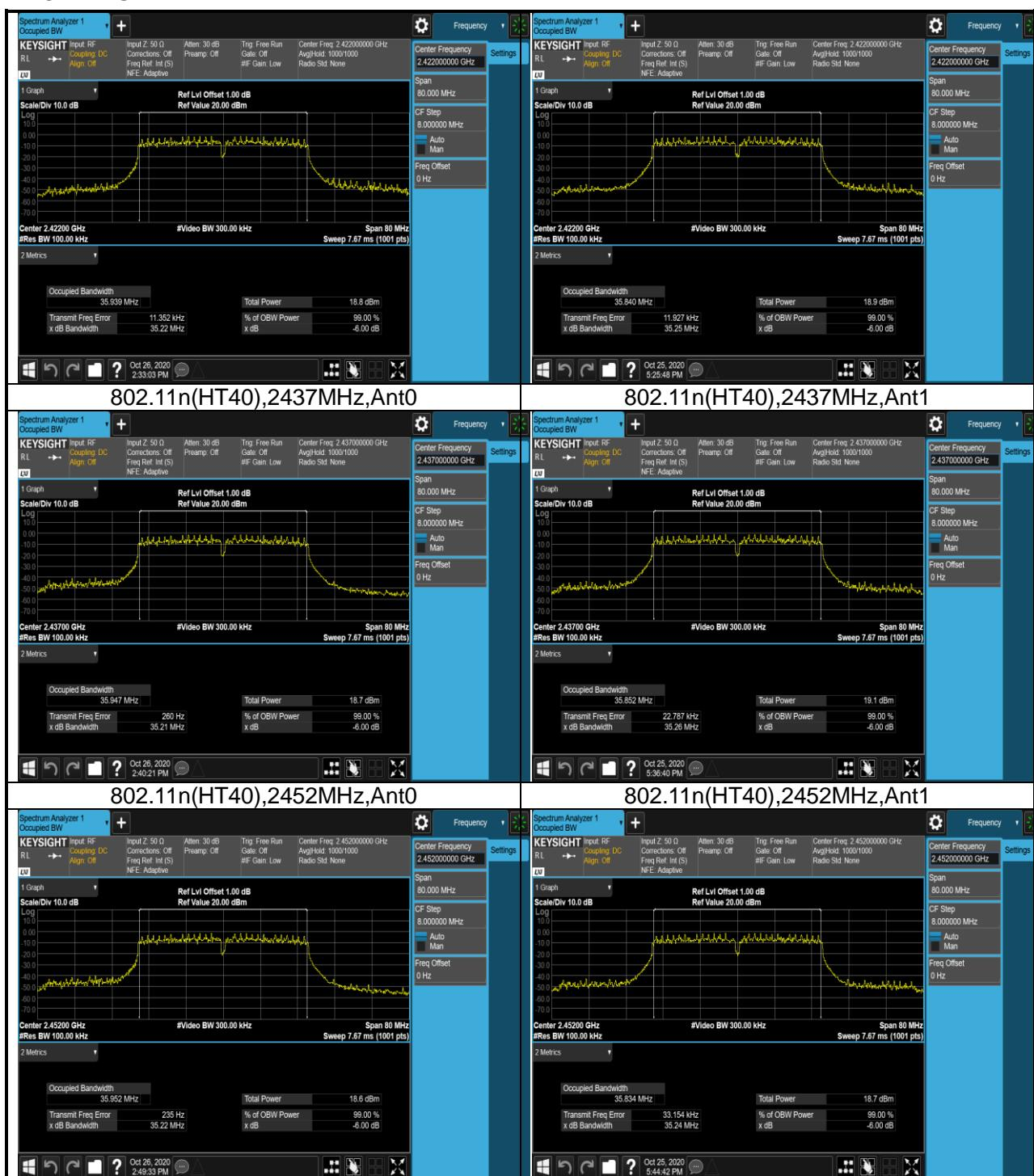
**TEST REPORT****3. Occupied Bandwidth****3.1 Test Data**
