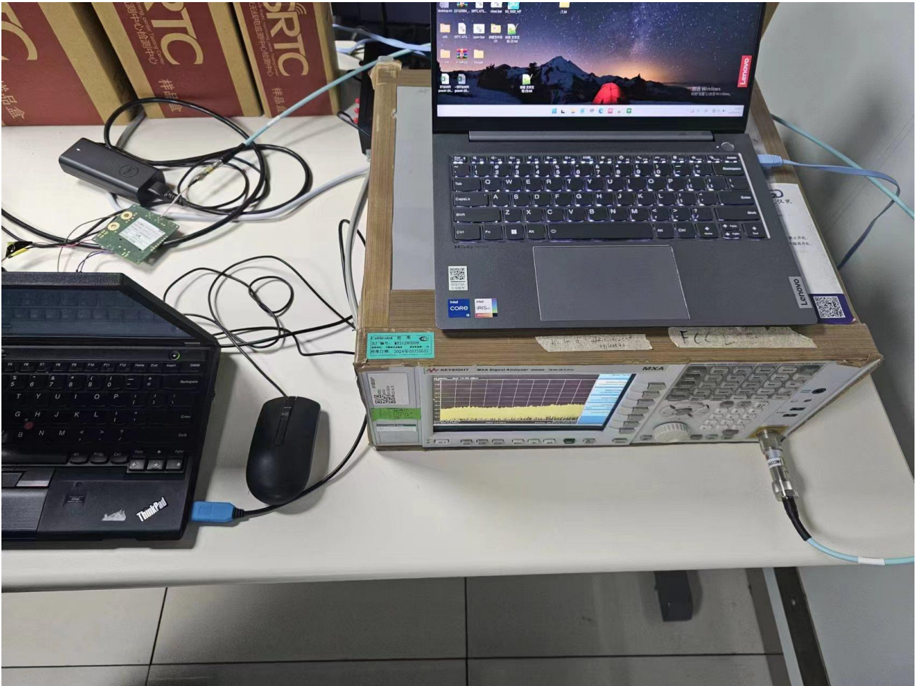
RF Conducted Test setup (BT/WIFI)
