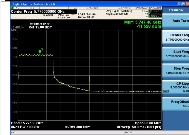
Mode:802.11ax HE80 Tone:242T Frequency:5775MHz Ant:Chain0
