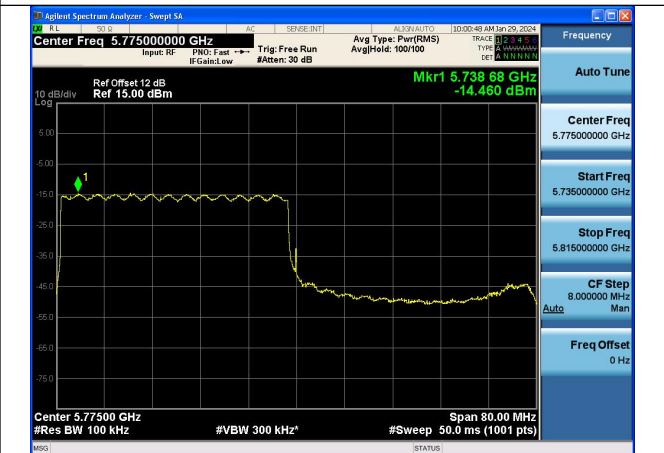
Mode:802.11ax HE80 Tone:484T Frequency:5775MHz Ant:Chain1
