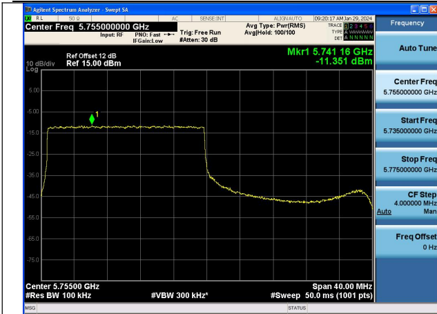
Mode:802.11ax HE40 Tone:242T Frequency:5755MHz Ant:Chain0
