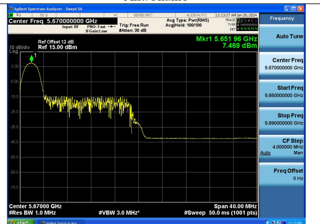
Mode:802.11ax HE40 Tone:26T Frequency:5670MHz Ant:Chain1
