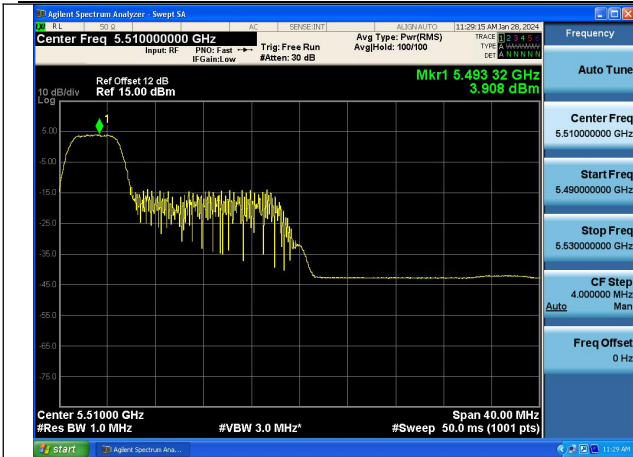
Mode:802.11ax HE40 Tone:52T Frequency:5510MHz Ant:Chain0
