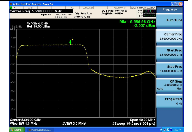
Mode:802.11ax HE40 Tone:242T Frequency:5590MHz Ant:Chain0
