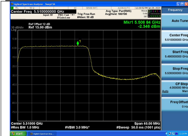
Mode:802.11ax HE40 Tone:242T Frequency:5510MHz Ant:Chain0
