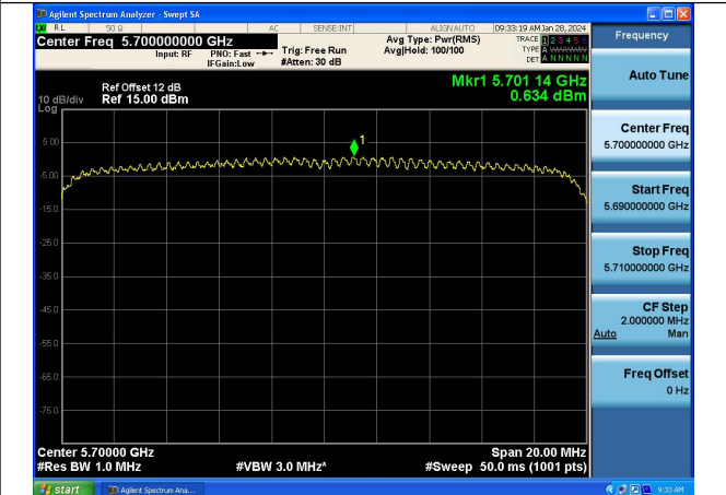
Mode:802.11ax HE20 Tone:242T Frequency:5700MHz Ant:Chain1
