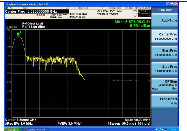
Mode:802.11ax HE40 Tone:26T Frequency:5590MHz Ant:Chain0
