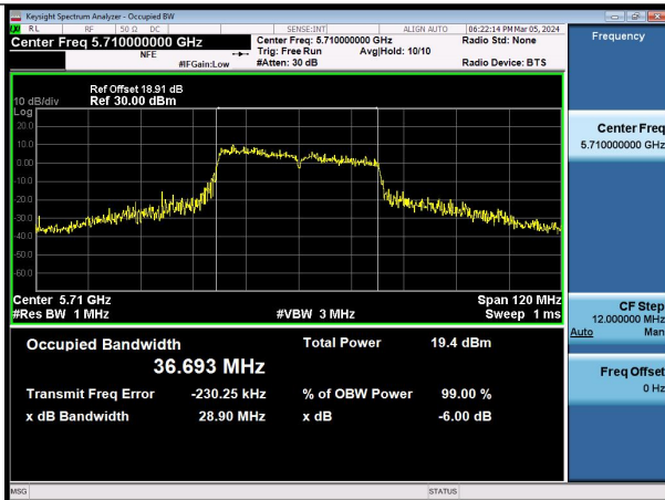
Mode:802.11ac VHT40 Frequency:5710MHz Ant:Chain0 scope:NII2C
