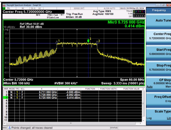
Mode:802.11ac VHT20 Frequency:5720MHz Ant:Chain0 scope:NII2C
