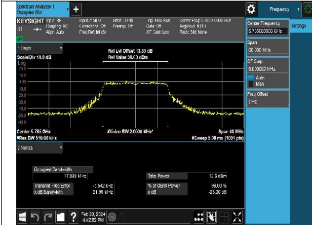
Mode:802.11n HT20 Frequency:5785MHz Ant:Chain1
