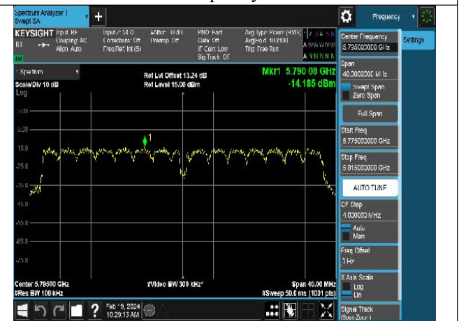
Mode:802.11n HT40 Frequency:5795MHz Ant:Chain1
