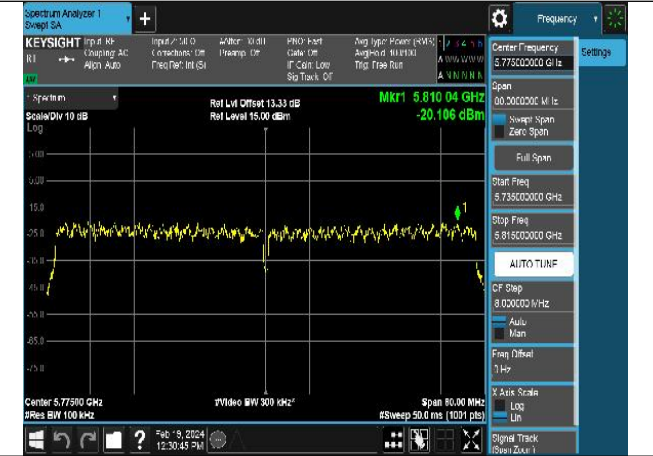
Mode:802.11ac VHT80 Frequency:5775MHz Ant:Chain1
