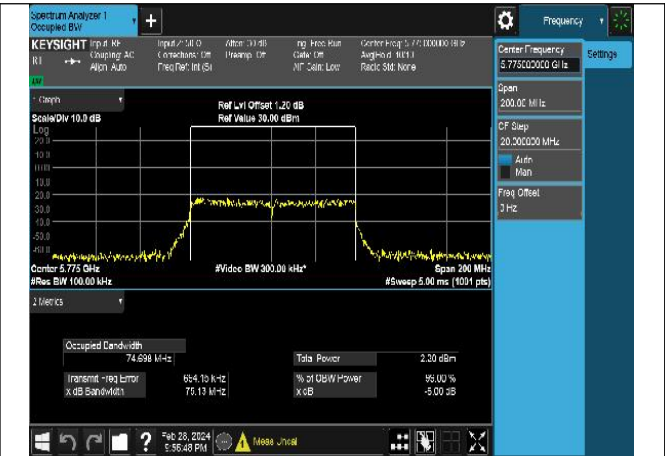
Mode:802.11ac VHT80 Frequency:5775MHz Ant:Chain1
