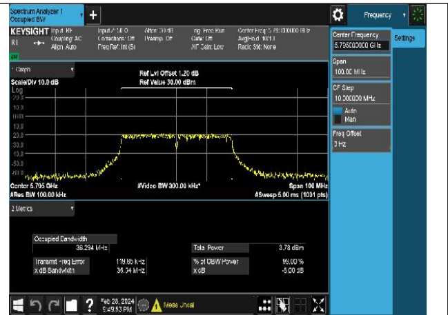
Mode:802.11ac VHT40 Frequency:5795MHz Ant:Chain0
