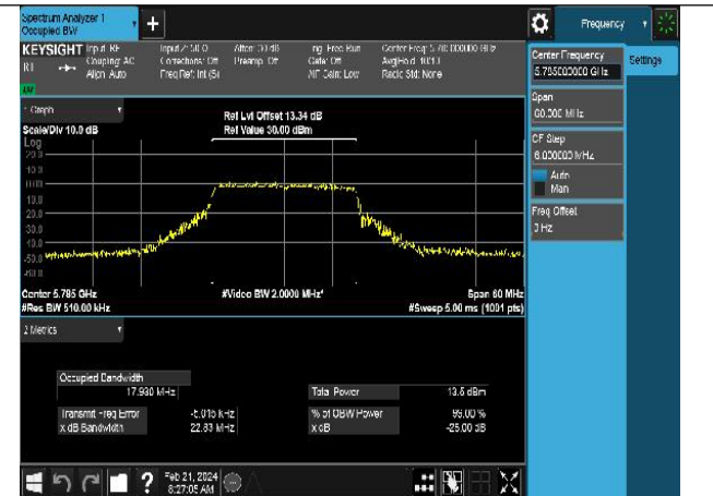
Mode:802.11ac VHT20 Frequency:5785MHz Ant:Chain0
