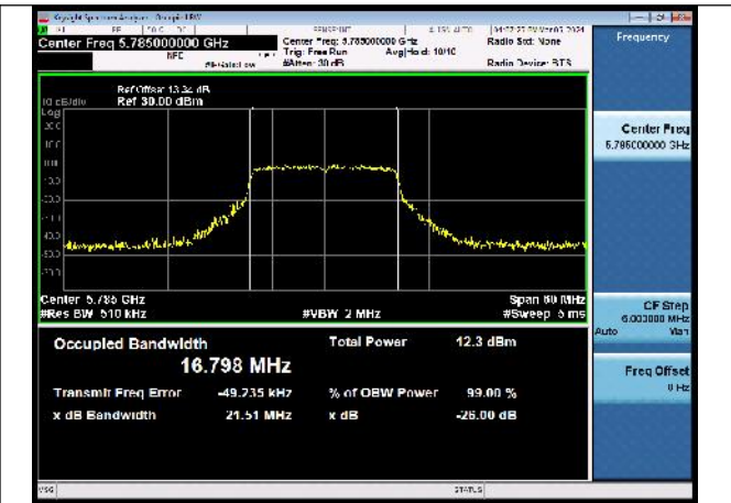
Mode:802.11n HT20 Frequency:5785MHz Ant:Chain0
