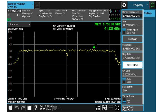
Mode:802.11ac VHT20 Frequency:5745MHz Ant:Chain1
