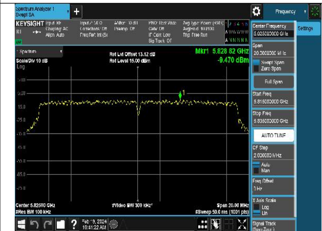
Mode:802.11ac VHT20 Frequency:5825MHz Ant:Chain1
