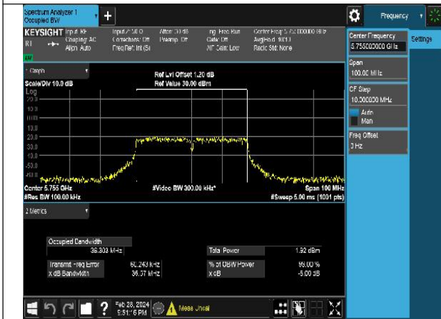
Mode:802.11ac VHT40 Frequency:5755MHz Ant:Chain1
