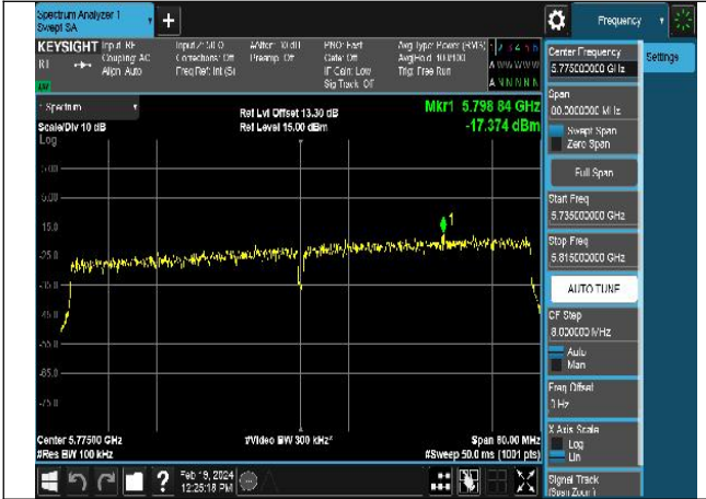
Mode:802.11ac VHT80 Frequency:5775MHz Ant:Chain0
