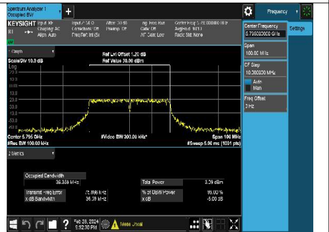
Mode:802.11ac VHT40 Frequency:5795MHz Ant:Chain1
