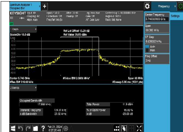
Mode:802.11ac VHT20 Frequency:5745MHz Ant:Chain0
