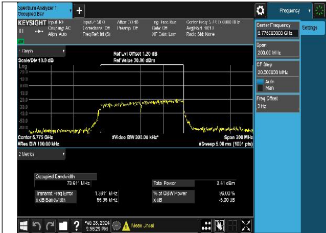
Mode:802.11ac VHT80 Frequency:5775MHz Ant:Chain0
