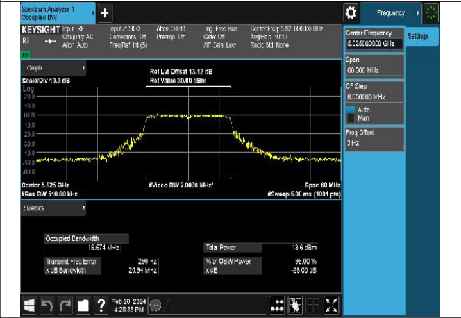
Mode:802.11a Frequency:5825MHz Ant:Chain1
