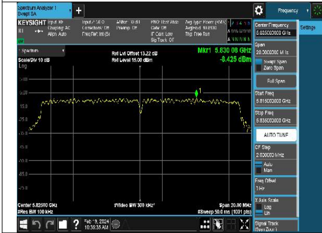
Mode:802.11ac VHT20 Frequency:5825MHz Ant:Chain0
