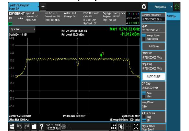
Mode:802.11a Frequency:5745MHz Ant:Chain1
