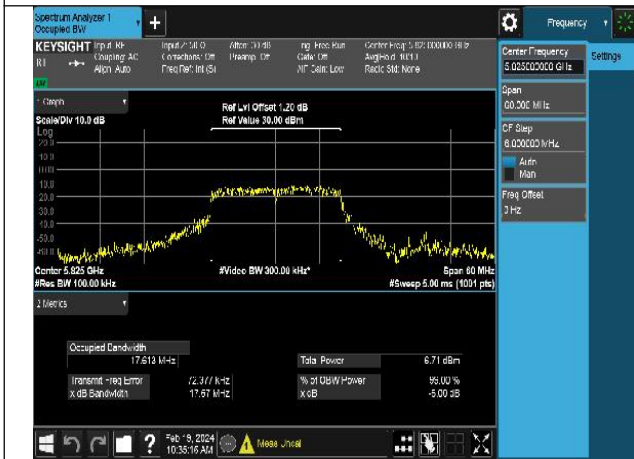
Mode:802.11ac VHT20 Frequency:5825MHz Ant:Chain0
