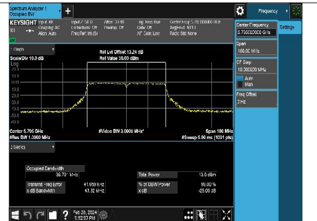
Mode:802.11ac VHT40 Frequency:5795MHz Ant:Chain1
