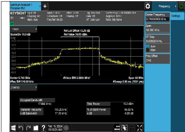
Mode:802.11n HT20 Frequency:5745MHz Ant:Chain0
