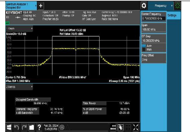
Mode:802.11ac VHT40 Frequency:5795MHz Ant:Chain0
