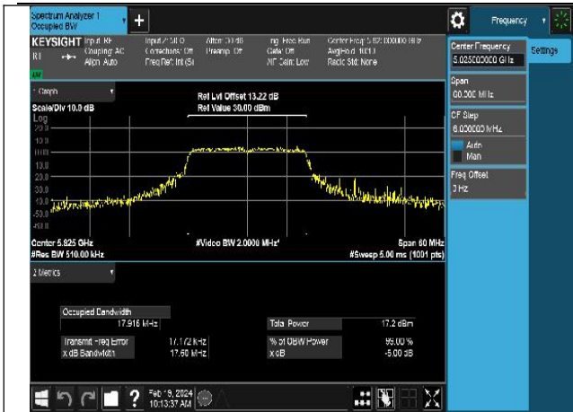
Mode:802.11n HT20 Frequency:5825MHz Ant:Chain0
