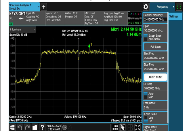
Mode:802.11n HT20 Frequency:2412MHz Ant:Chain1
