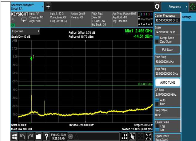
Mode:802.11b Frequency:2462MHz Ant:Chain0
