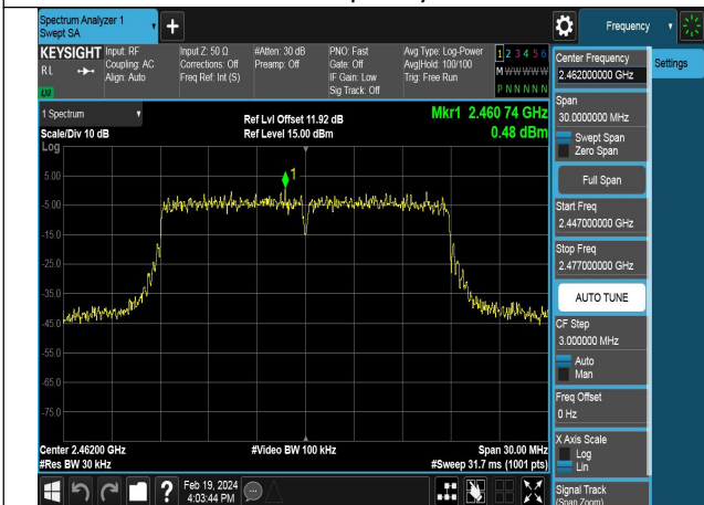
Mode:802.11n HT20 Frequency:2462MHz Ant:Chain0
