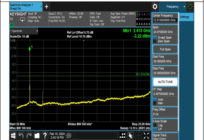
Mode:802.11b Frequency:2412MHz Ant:Chain1
