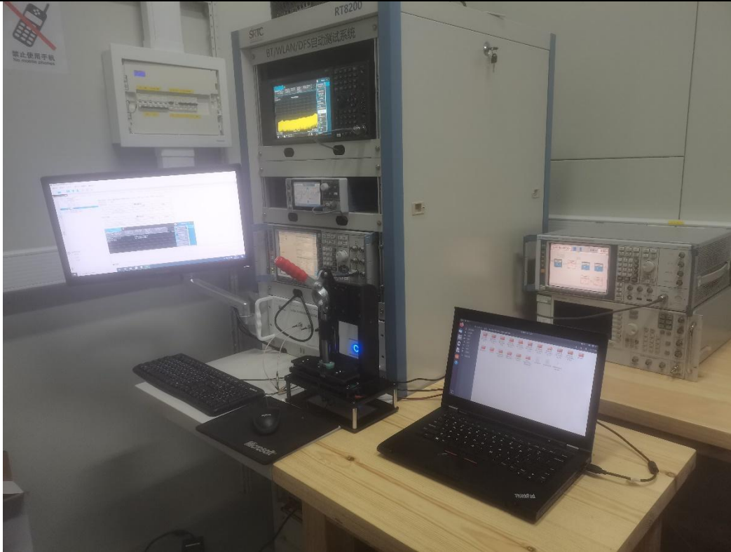
RF Conducted Test setup (DFS)
