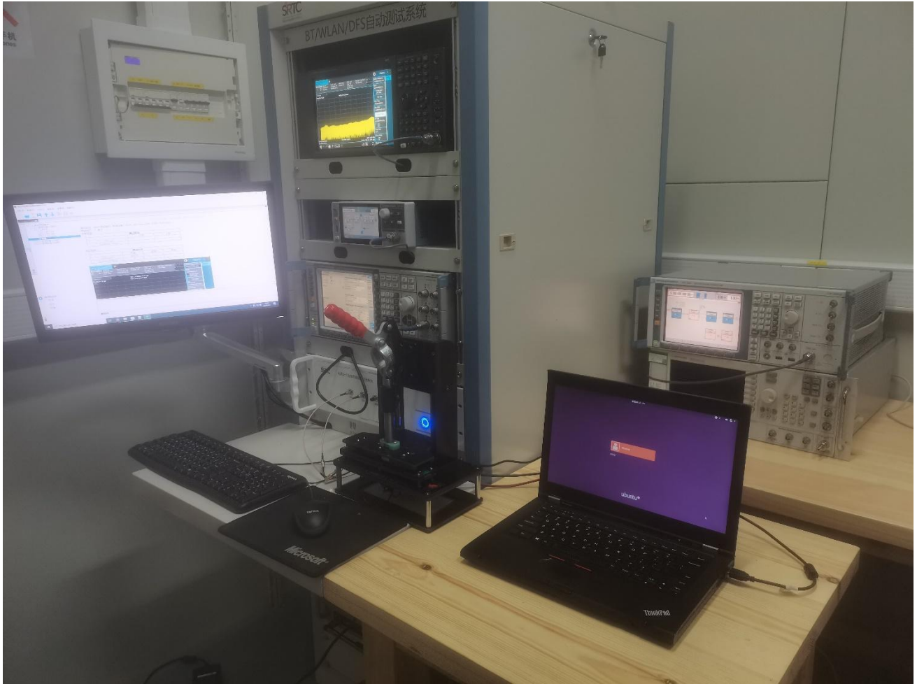
RF Conducted Test setup (BT/WIFI)
