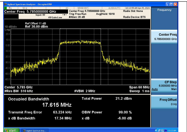
Mode:802.11ac VHT20 Frequency:5785MHz Ant:Chain0
