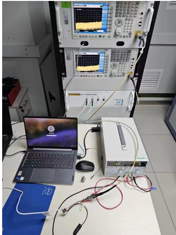
RF Conducted Test setup (BT/WIFI)
