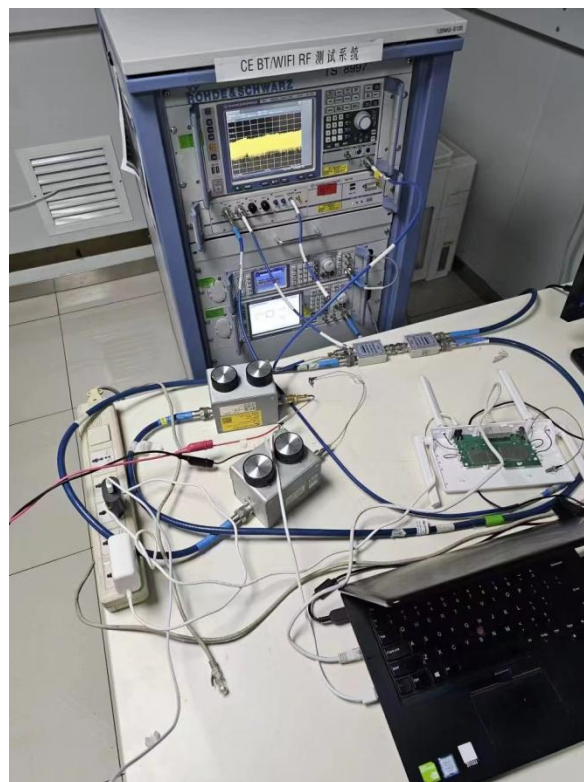
RF Conducted Test setup (DFS)
