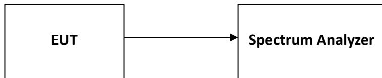
**1.19 Test Results of Maximum conducted output power**
