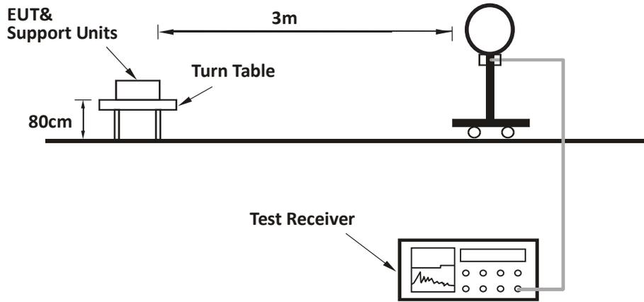
For Radiated emission 30MHz to 1GHz:
