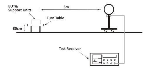
For Radiated emission 30MHz to 1GHz:
